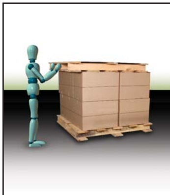
1. Add replacement pallet or slip sheet to top of load.
