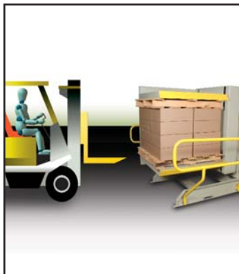
2. Place loaded pallet into inverter.
