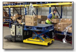
The Walkie can support all types and sizes of skids and pallets, including GEO and half pallets
